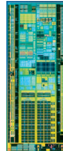
Intel® Atom™ processor Initial clock speed: 1.86GHz Transistors: 47 million Manufacturing technology: 45nm
