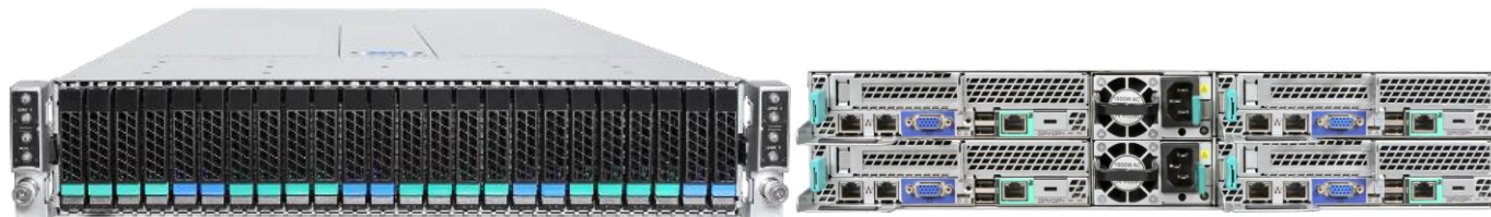
Figure 6. Intel® Server Chassis H2224XXKR2 w/ 4 Nodes + 2 PSUs Installed
