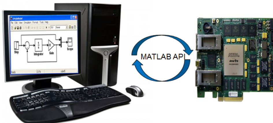
Figure 128. Hardware in the Loop Host-Target Setup
