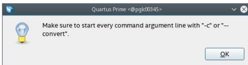
Figure 11. Error message when command argument lines do not begin with -c or --convert
