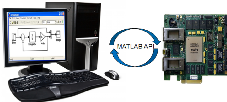
Figure 20. Hardware in the Loop Host-Target Setup
